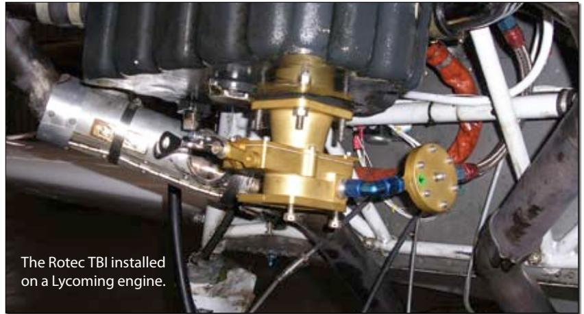
body throat. At full power, the slide is fully retracted, allowing maximum airflow and exposing all of the holes in the fuel-metering tube. At idle, the slide is extended, closing off the throat opening and reducing the number of metering-tube holes that are exposed to airflow. Fuel mixture is controlled by rotating the metering tube through 90° of rotational travel via a control arm that's connected to a simple push-pull control.
